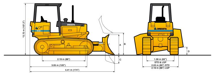
$<sup>^{\</sup>star}$  Dimension includes 53.6 mm (2.11") grouser height Overall height with Cab ROPS – 2.76 m (108.5")
